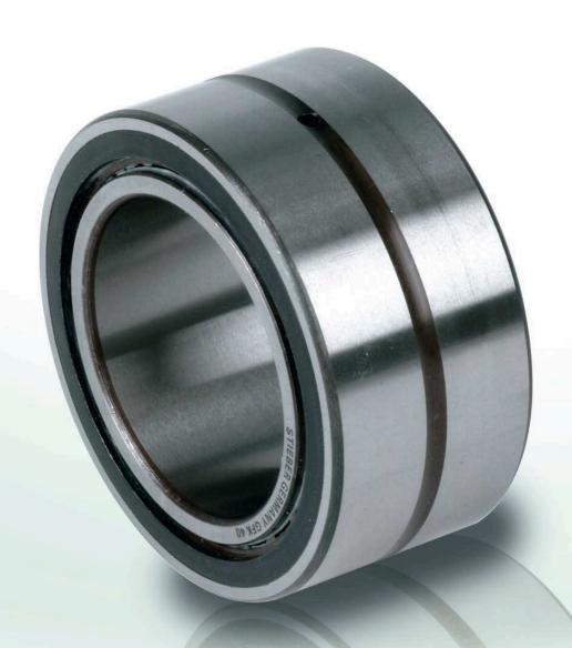
ype GFK is a sprag type freewheel integrated into a 59.. series ball bearing. This design provides high torque capacity for minimal outside diameter. It is a bearing supported type, delivered grease lubricated.
